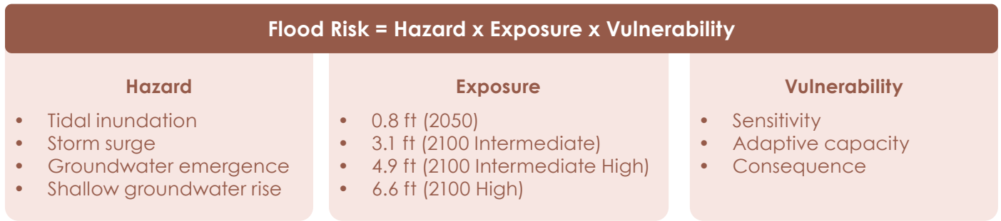
Figure 1–9. A description of flood risk for the RSAP. This includes the minimum coastal flood hazards, exposure due to minimum sea level rise scenarios, and components of vulnerability. For more information on types of flood hazards, see Coastal Flood Hazards and Sea Level Rise Scenarios Standard (Section 3.3.1).
