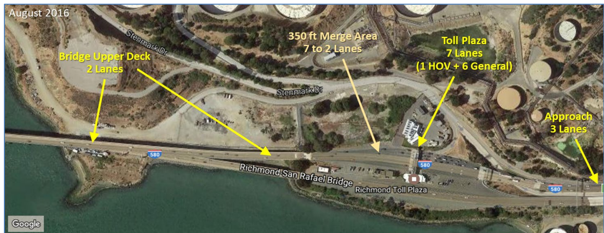
Figure 2-3: Initial Conditions – Westbound Bridge Approach in Richmond
