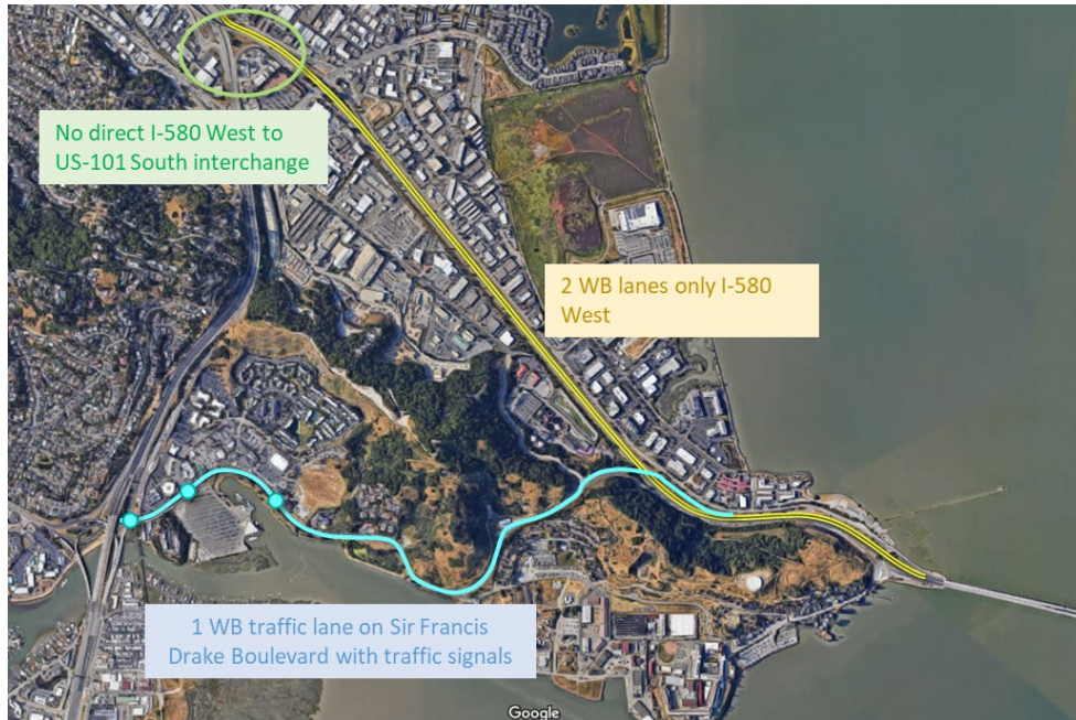
Figure 8-85: Marin County Roadway Configuration Constraints
