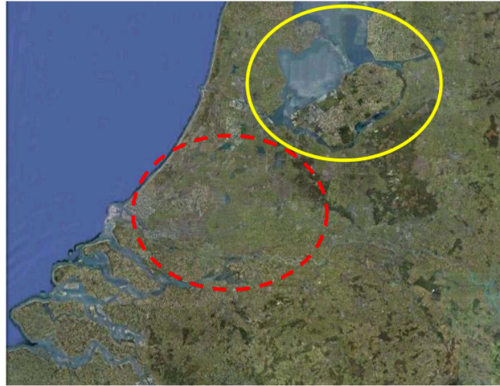
Figure 2. An area with traditional polders (red, dotted circle) and area with modern polders (yellow circle).
