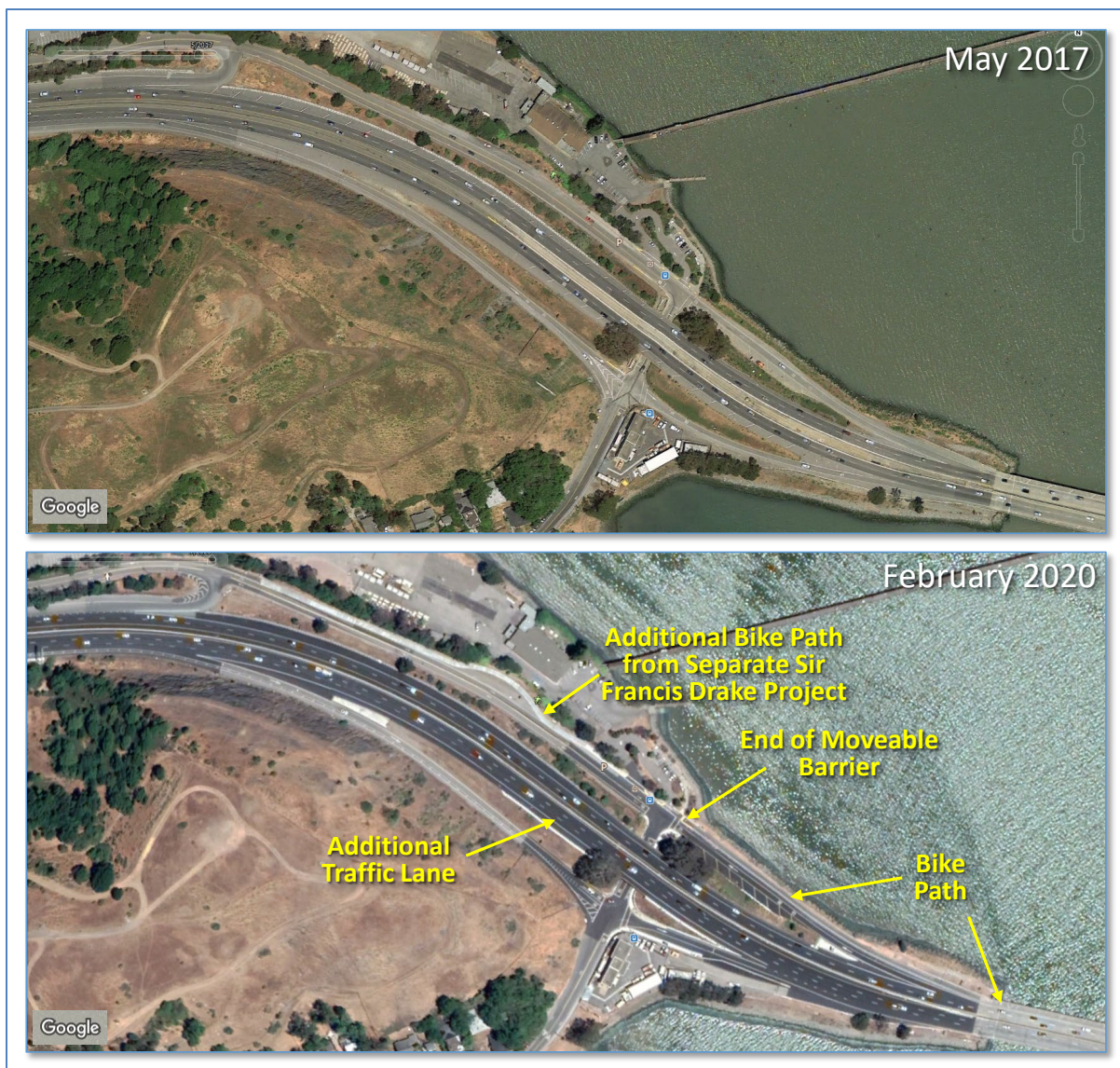
Figure 2-19: Modifications of Marin County Approach
