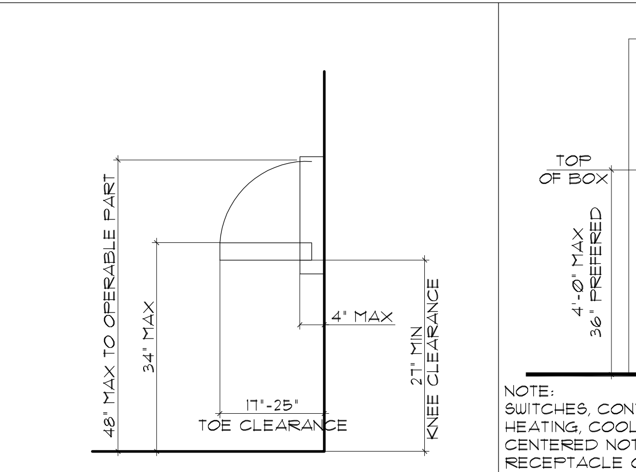
9 BABY CHANGING STATION DETAIL SCALE: 3/4"=1'-0"
