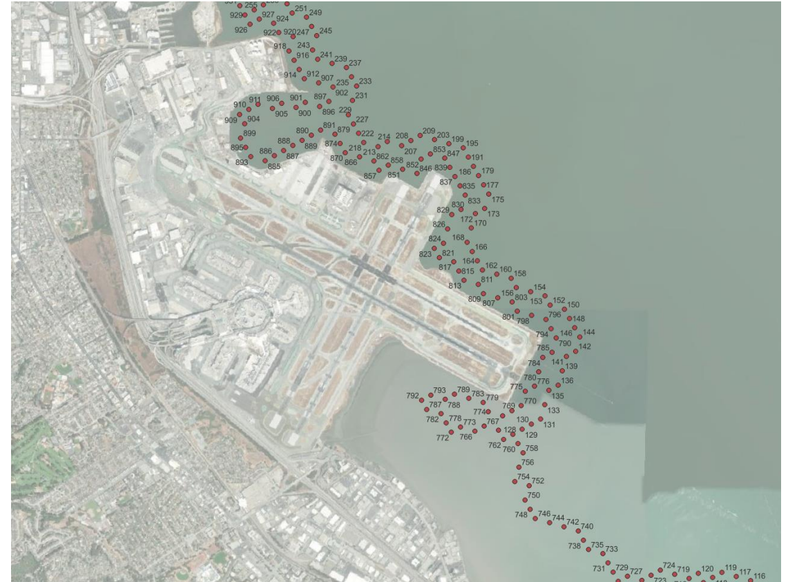
Passpoints along SFO Shoreline where surge and wave time series data are available
