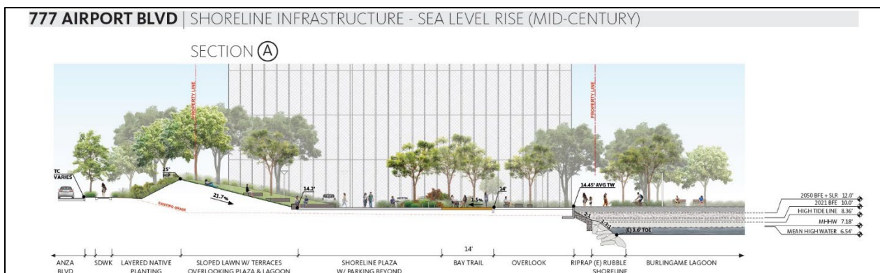
Figure 5: Section diagram of shoreline elevations and projected sea level rise through 2050.
